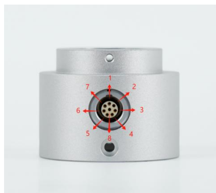
Figure 2 Physical Diagram of Aviation Plug
