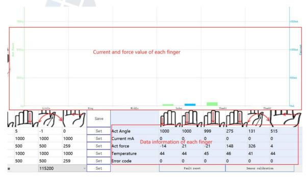
If the force applied to a finger is not accurate, the force sensor should be calibrated.
