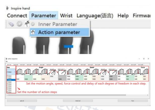
This software can set the 1st to 13th set of action sequence data in the dexterous hand. Each set of action sequences has up to 8 steps of motion. The finger angle, motion speed, magnitude of force, and waiting time for each step can be set separately.
