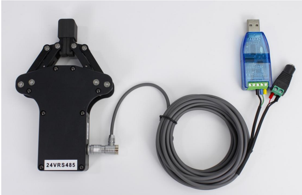
RS485 Interface Connection
